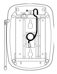
4. Insert the supplied AC adapter's barrel plug into the **DC IN 9V** jack on the back of the base.
